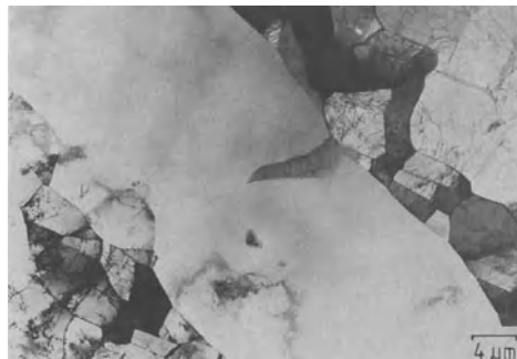
Fig. 4.40 Deformation bands containing subgrains formed in large grain. Sample taken from position A in billet, at location 2 on load/displacement curve. Selected area diffraction patterns from the three areas indicated that all have zone axis very close to \langle 112 \rangle but the central band is rotated by 33^\circ about this axis with respect to its neighbours.
