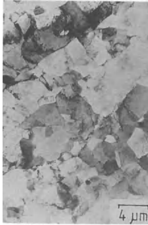
Fig. 4.42 Equiaxed subgrains within deformation bands in sample taken from the same position as that in Fig. 4.41 but at location 6 in the load/displacement curve when steady-state deformation is attained.
