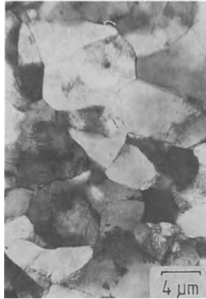
Fig. 4.45 Typical subgrain and dislocation structure observed during steady-state extrusion. Sample taken from position B in billet at location 7 in load/displacement curve.
