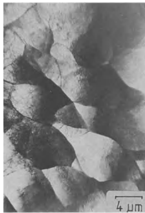
Fig. 4.41 Elongated subgrains containing very high dislocation density observed at mouth at peak pressure. Dynamic recovery is incomplete.
