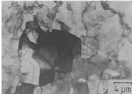
Fig. 4.44 Specimen taken from the back of the billet at location 6 in the load/displacement curve. Deformation in this zone is still limited although steady-state deformation has essentially been attained.
