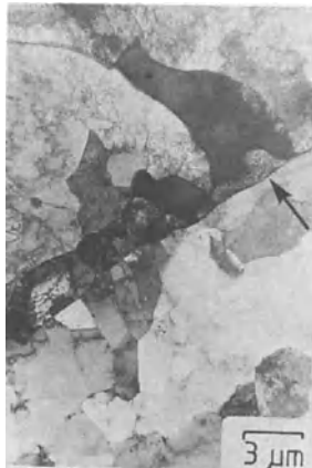
Fig. 4.43 Sample containing high-angle grain boundary (arrowed) taken from the same location and position in the load/displacement curve as Fig. 4.42. Comparison of Figs. 4.42 and 4.43 shows that once steady-state deformation is achieved the microstructure becomes much more uniform.
