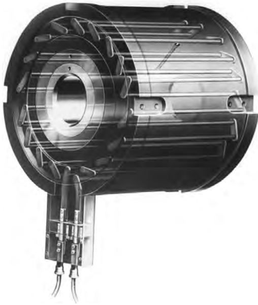
Fig. 1.12 Three-piece container with induction heating
