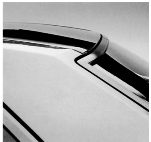
Fig. 2.22 Rear window frame of the Mercedes W124 manufactured from extruded aluminum sections. The front windshield of the vehicle had a similar frame. Source: Erbslöh
