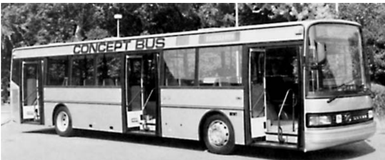
Fig. 2.31 The study of a coach presented at IAA 1987 with bolted, supporting lattice frame construction in extruded aluminum sections. Source: Alusuisse
