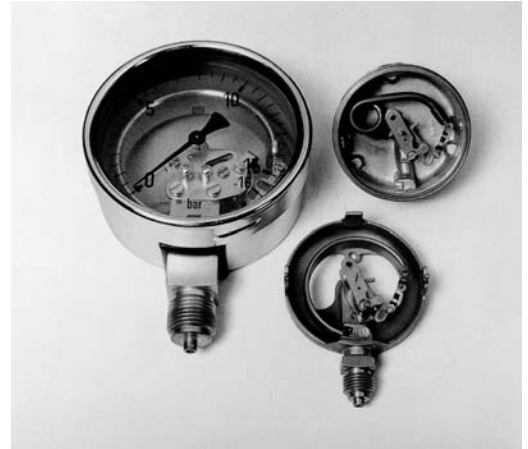
Fig. 2.88 Manometer springs in extruded and drawn tin-bronze tubes. Source: Wieland-Werke AG
