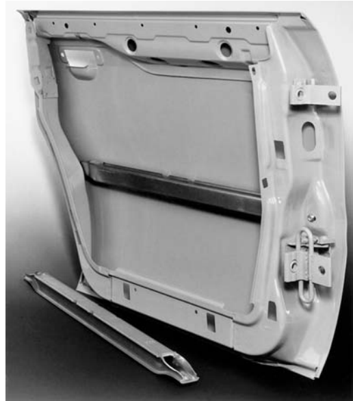
Fig. 2.24 Side door of the Audi 100 with built-in chromated for corrosion protection, extruded section in the aluminum alloy AlMgSi1, F 31 with R_{p0.2} = 260 \text{ N/mm}^2 and A_5 = 10\% . Source: Aluisse
