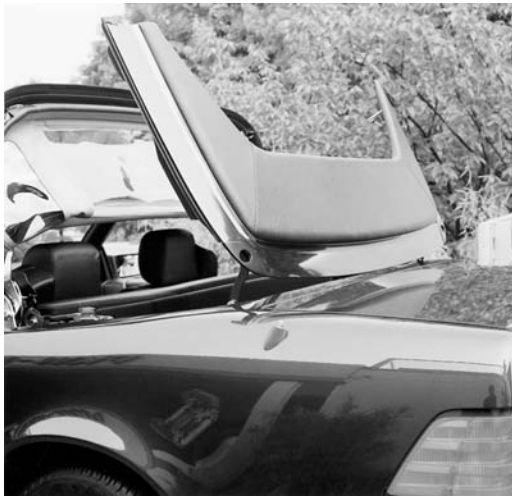
Fig. 2.23 Hood container cover of the Mercedes 300 SL and 500 SL class with extruded aluminum section frames. Source: Erbslöh
