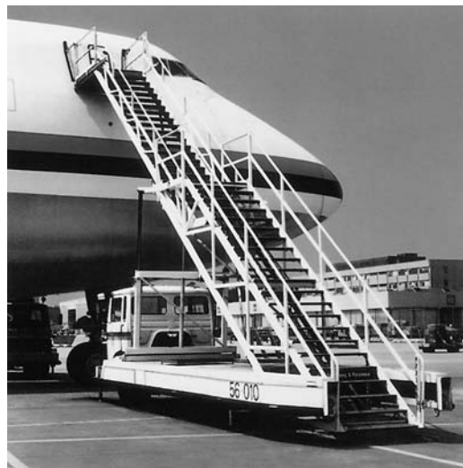
Fig. 2.70 Movable stairs for embarkation and disembarkation from aircraft at airports manufactured in extruded aluminum sections. Source: Alusuisse
