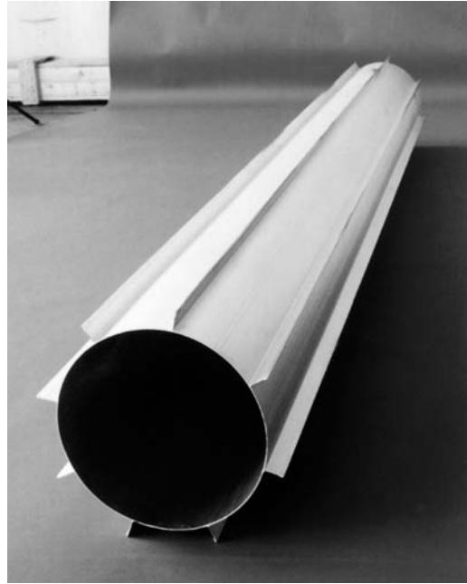
Fig. 2.42 Extruded tube with integral stringers in the aluminum alloy AA6013. Source: Daimler Benz Aerospace Airbus
