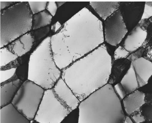
Fig. 4.42 Subgrain formation in Al99.99 (hot strip). The width is approximately 8.4 \mu\text{m} [Grz 93]
