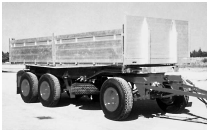
Fig. 2.37 Trailer with planked construction and chassis in extruded aluminum sections. Source: Alusuisse
