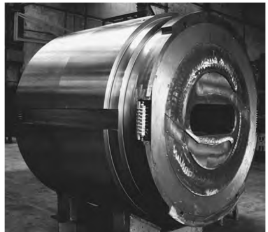
Fig. 7.95 Container with oval bore for direct extrusion of aluminum alloys for a 75 MN extrusion press. Source: Aluisse
