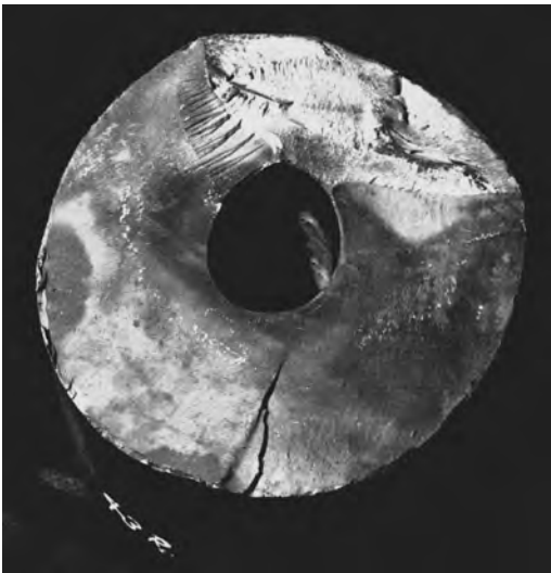
Fig. 7.94 Failed extrusion stem for indirect extrusion. Source: SMS Schloemann
