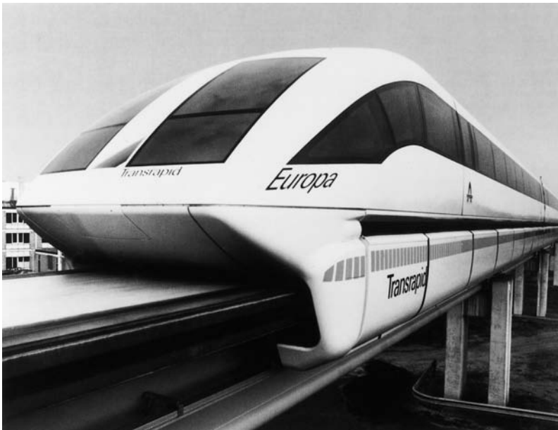
Fig. 2.16 Prototype of the magnetic levitation Transrapid manufactured with bolted aluminium large profile technology using aluminium AlMgSi0.7 extruded sections. Source: Alusuisse
