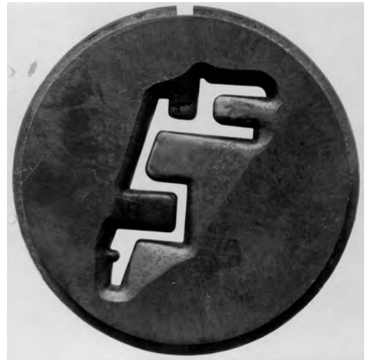
Fig. 7.24 Extrusion die with different-length tapered inlets to the die aperture for the production of a steel section. Source: Krupp-Hoesch
