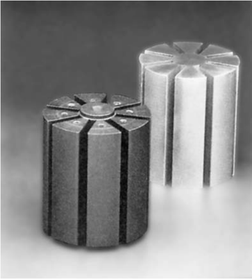
Fig. 2.54 Extruded blanks in AlMgSi0.5 for rotors of the air compressor of a pneumatic tanker pumping unit for sewage. Source: Honsel
