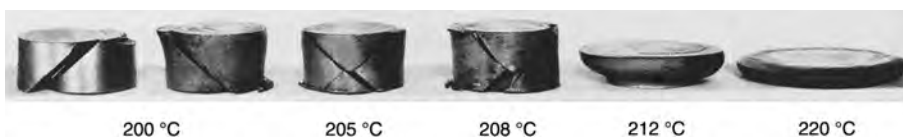
Fig. 5.9 Deformation behavior of the magnesium alloy MgAl6Zn in hot-compression tests in the temperature range between 200 and 220 °C (Source: Schmidt/Beck)
