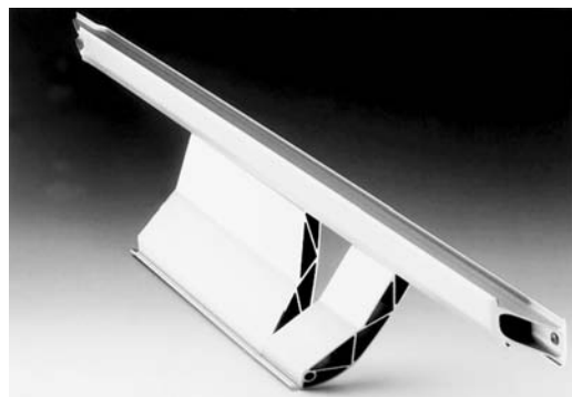
Fig. 2.25 Side-impact beam from the Audi 8 consisting of two extruded sections. Alloy AlMgSi1, F 31. The side-impact beam can be seen installed in Fig. 2.27. Source: Aluisse
