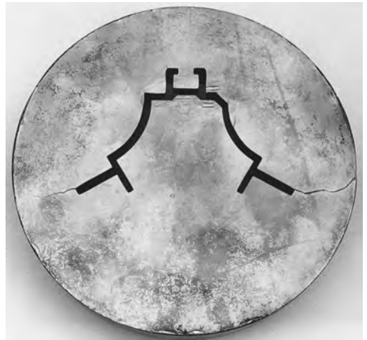
Fig. 7.115 Billet side of an extrusion die for the production of a brass section that has cracked at a critical cross section of the die aperture. Source: Wieland-Werke AG
