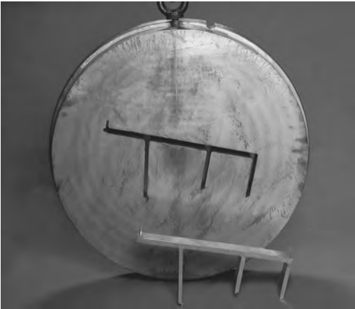
Fig. 7.48 Flat die for the production of the solid AlMgSi0.5 section shown in front of the die. Source: Alusuisse
