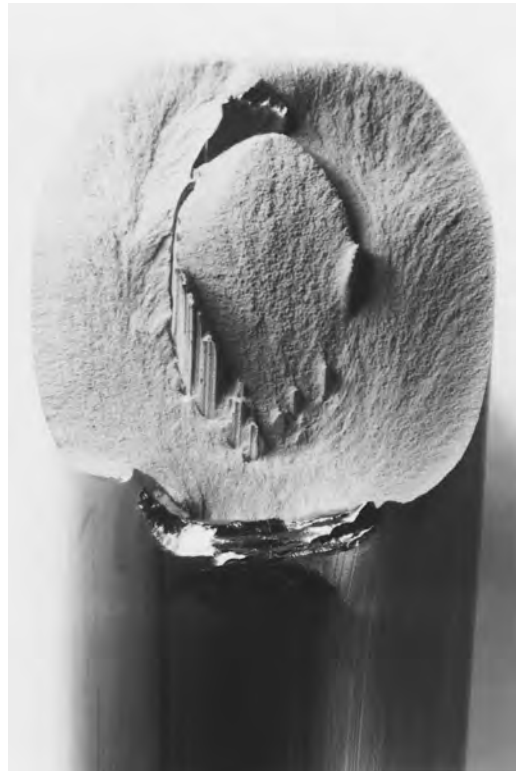
Fig. 5.46 Extrusion defect (piping) in \alpha - \beta -brass [Die 76]
