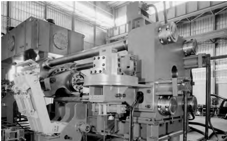
Fig. 6.13 16 MN aluminum alloy press with auxiliary equipment. (Factory assembly Danieli Breda)
