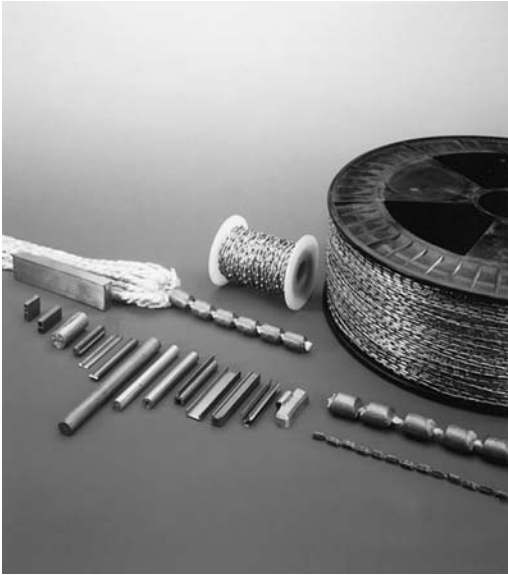
Fig. 2.3 Extruded solder with several flux cores, lead sheathed cable, and window spacer sections in lead alloys for double glazed windows, as well as lead lines for fishing nets and curtain weights. Source: Collin
