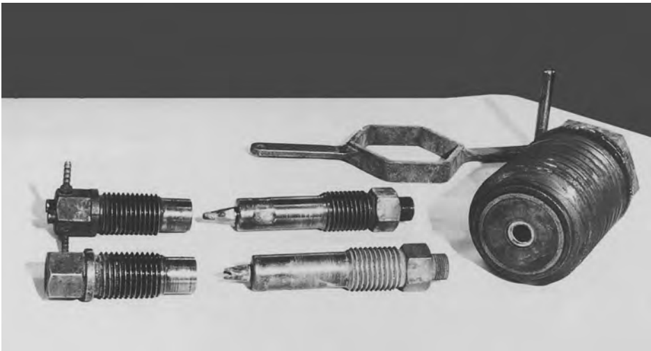
Fig. 5.7 Die holder, left, and hollow mandrel, right, as well as the front nut of the container with the pressure nut for adjusting the hollow mandrel (See Fig. 5.6) (Source: Collin, Alchacht)
