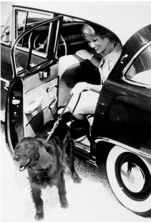
Fig. 2.21 Automobile window frame in extruded, age-hardened, and anodized aluminum sections on an Opel Rekord manufactured in 1958. Source: Opel
