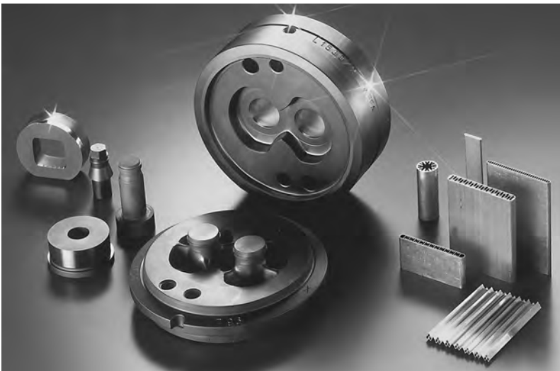
Fig. 7.127 Left, chemical vapor deposition (CVD)-coated aluminum extrusion dies. Right, demanding heat exchanger sections in AlMgSi0.5 produced with CVD-coated dies. Source: WEFA Singen GmbH
