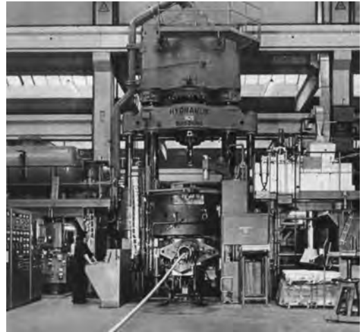
Fig. 3.87 30 MN cable sheathing press for aluminum [Rie 72]
