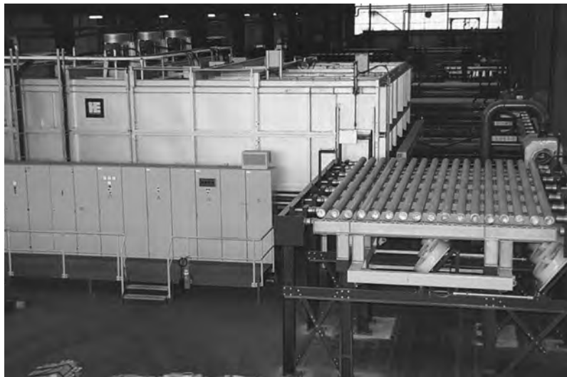
Fig. 6.79 Continuous homogenization plant for aluminum extrusion billets. Source: VAW-Elbeweke, Stade
