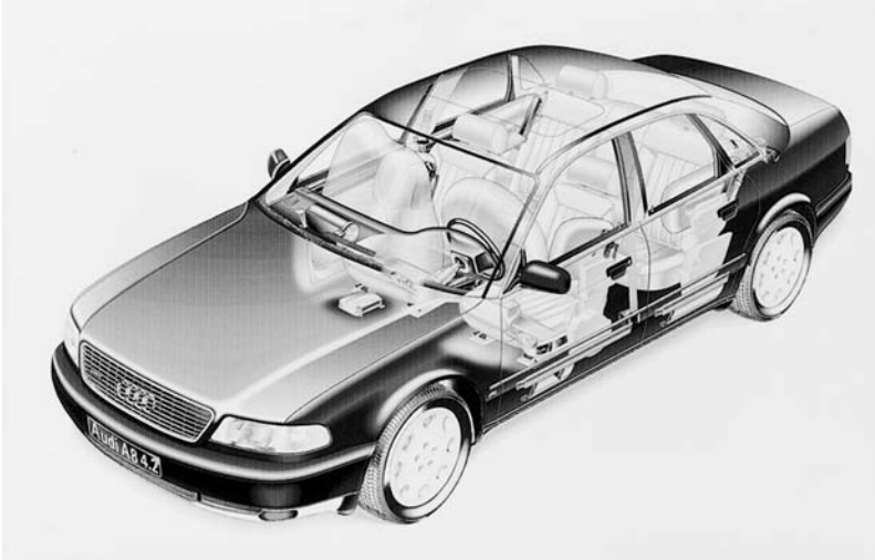
Fig. 2.27 Audi A8 Quattro with a body of age-hardened aluminum alloys using the Alcoa space frame concept. Source: Audi
