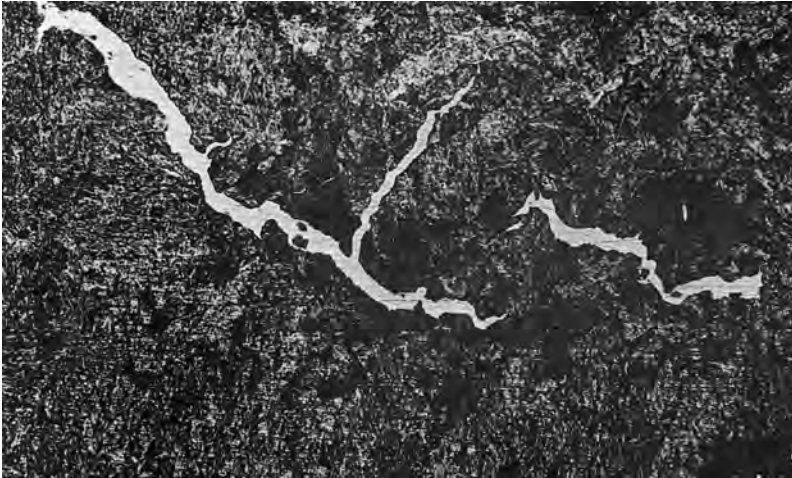
Fig. 7.122 Solder fracture in the liner of the container of an aluminum extrusion press with a 250 mm bore after a large number of extrusions with the bearing material AlSn6Cu1. The liner was manufactured in the hot working steel 1.2306.
