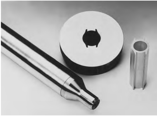
Fig. 7.73 Extrusion die and stepped mandrel for the production of the wristwatch housing section shown at right. Source: Wieland-Werke AG
