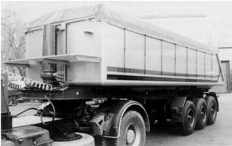
Fig. 2.36 Tipping trailer with covered body made entirely from extruded multicore hollow sections for the transport of fine powdered goods. Source: Alusuisse
