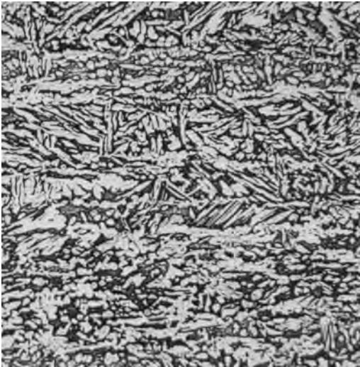
Fig. 5.43 Brass with acicular \alpha - \beta -structure, etched. Image width is approximately 0.275mm [Wie 86]
