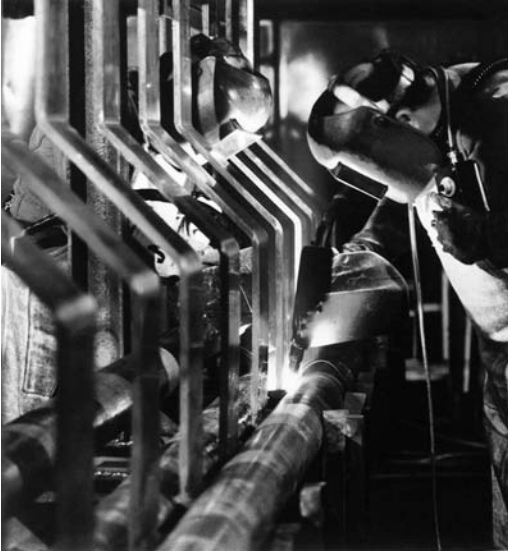
Fig. 2.76 Copper bus bars from extruded semifinished products. Source: KM-Kabelmetall AG
