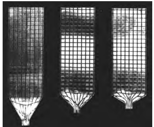
Fig. 3.59 Development of the deformation zone with different die opening angles for cold indirect extrusion with lubrication and without a shell of Al99.5
