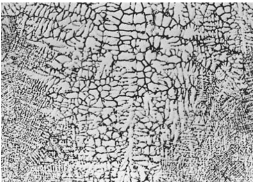
Fig. 4.22 Example of a cellular/dendritic solidified structure. The width is approximately 1.0 mm
