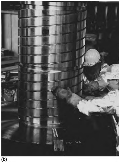
Fig. 7.98 (a) Combination heating and cooling system. Source: Groos. (b) Liner holder with cooling grooves. Source: Böhler
