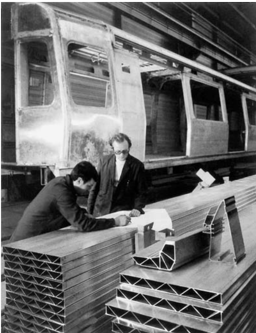
Fig. 2.9 Assembly of an aluminum MF77 type shell for the Paris Metro using welded large section technology together with some large sections ready for assembly. Source: Alusuisse
