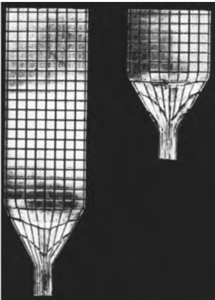
Fig. 3.58 Stages in indirect cold extrusion with lubrication and without a shell of Al99.5
