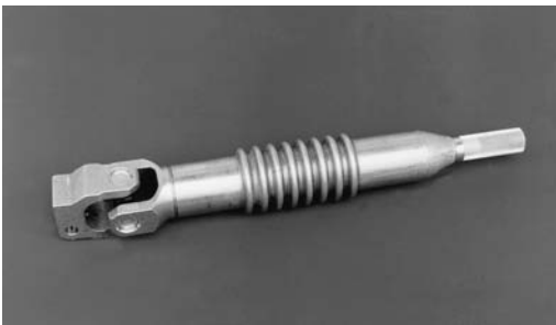
Fig. 2.26 Steering link in the alloy AlMgSi1, F 31. The connection on the left-hand side is from an extruded section, whereas the round, easily deformed in the event of a crash, corrugated section with the transition to the steering column was manufactured from an extruded tube. The corrugated region is heat treated to a strength of F 22 to F 25. Source: Aluisse
