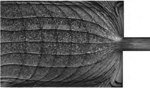
Fig. 3.8 Stage in hot direct extrusion of AlMg3 without lubrication and without a shell (container diam = 140 mm; extrusion ratio V = 50 ; initial billet length = 450 mm; initial billet temperature = container temperature = 450 °C)
