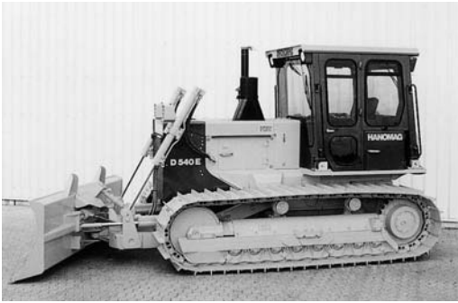
Fig. 2.91 Special sections as guide plates, guide wheels, scraper edges, and stringers for construction machinery. Source: Krupp-Hoesch
