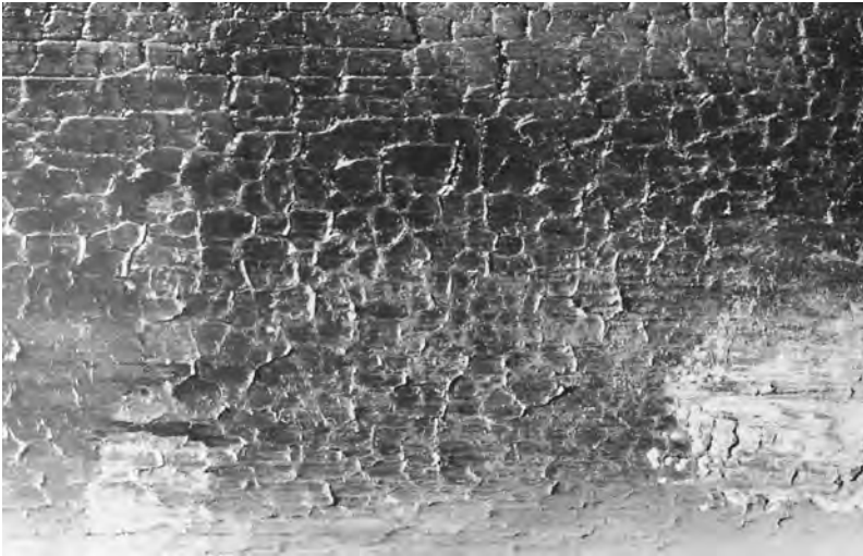
Fig. 7.119 Hot cracking network on the working surface of a tapered extrusion mandrel in the hot working steel 1.2367 for the production of copper tubes, resulting from the fluctuating tensile and compressive stresses. Copper that has welded to the mandrel surface can be seen in the lower right and left areas of the photograph. Source: Wieland-Werke AG
