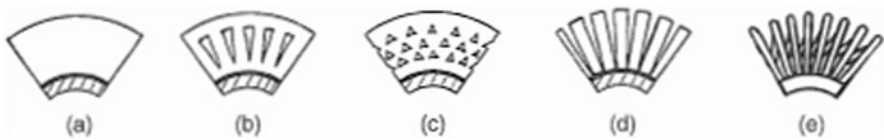
Fig. 4.22 Enhanced circular fin geometries: (a) plain circular fin; (b) slotted fin; (c) punched and bent triangular projections; (d) segmented fin; (e) wire loop extended surface (Webb 1987)
