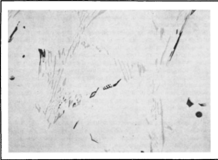
Fig. 5. 3003 as-cast ingot showing the distribution of predominantly (Mn,Fe)Al_6 (light) and (Fe,Mn)_3SiAl_{12} (dark) at dendrite interstices. 10% phosphoric acid, 455 \times . (Courtesy of Kaiser Aluminum & Chemical Corp.)
