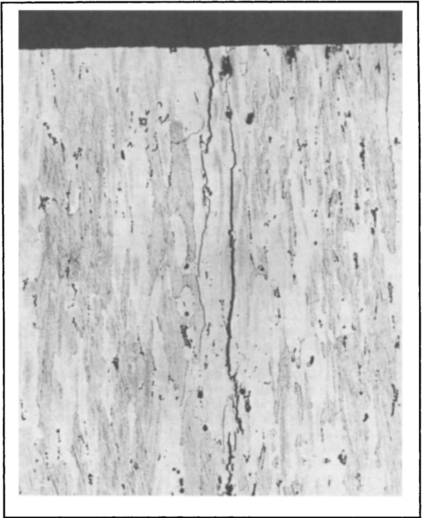
Fig. 4. Typical intergranular stress corrosion crack in 6.4-mm (0.25-in.) 7075-T651 plate stressed in short transverse direction. (Courtesy of Alcoa Laboratories)
