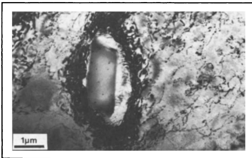
Fig. 55. Region of high local deformation in the vicinity of a coarse \text{FeAl}_3 particle in a cold rolled sample (20% reduction). (Courtesy of Alcan International Ltd.)
